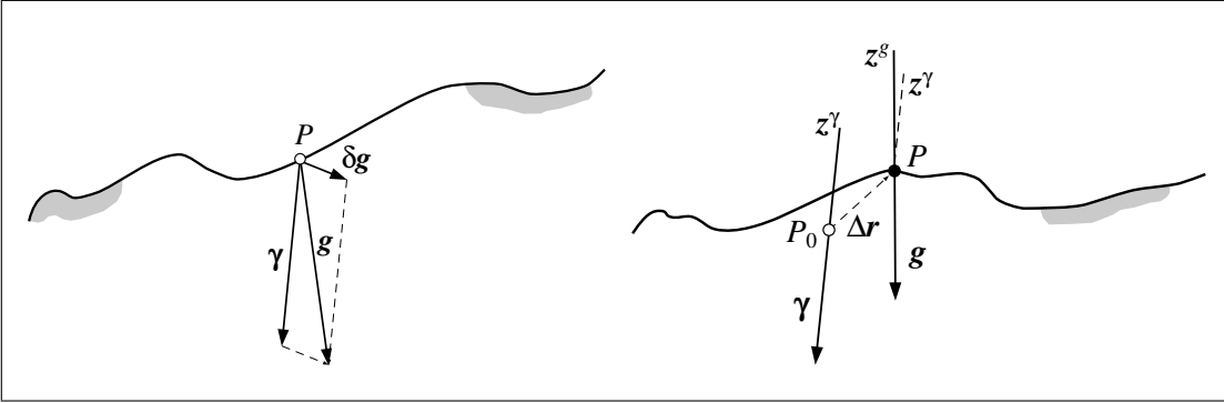
Figure 8.2.: Definition of gravity disturbance (left) and gravity anomaly (right).
