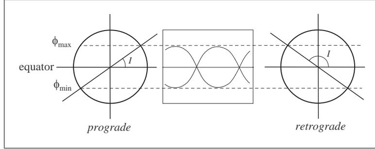
**Figure 2.7.:** The inclination determines the maximum and minimum latitude that ground-tracks can attain:  $\phi_{\min}$ ,  $\phi_{\max}$ .
