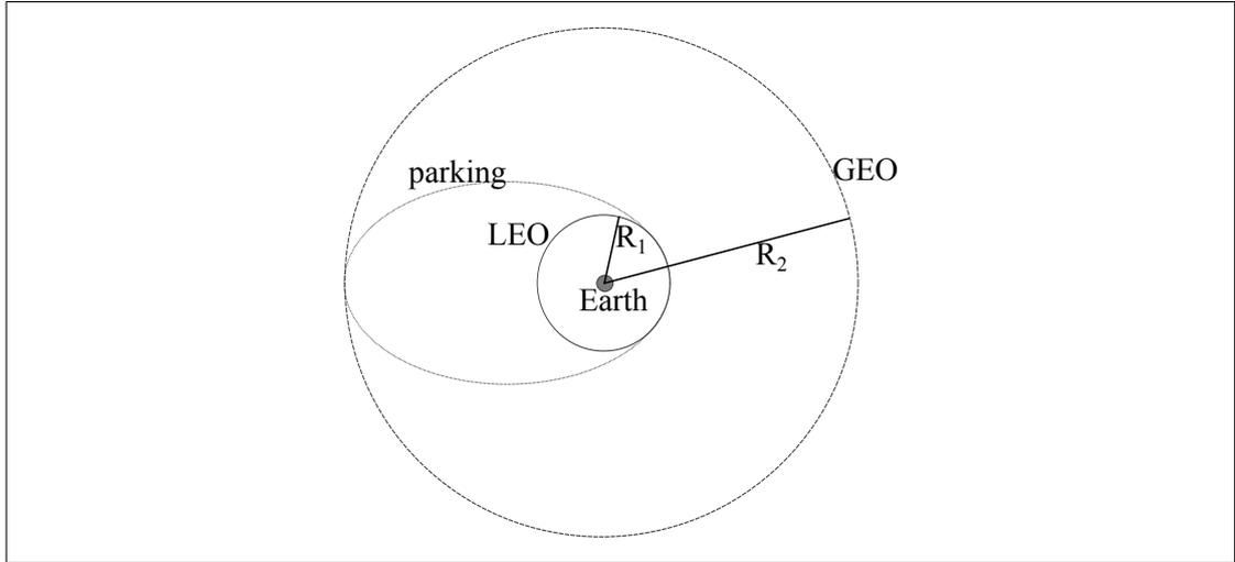
**Figure 2.12.:** Hohmann transfer between two circular orbits.
