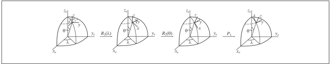
**Figure B.3.:** Transformation of the global Earth-fixed system into the local North oriented system.
