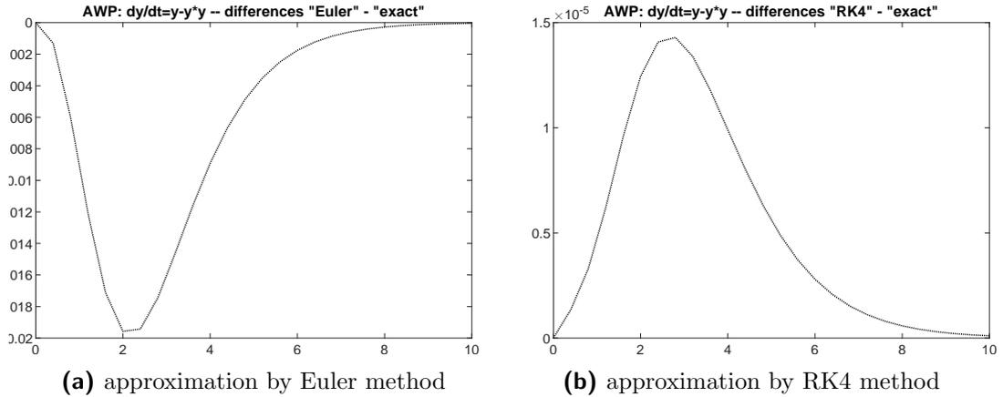
**Figure C.2.:** Differences between the numerical approximation and the exact solution for the ODE  $y' = y - y^2$ .
