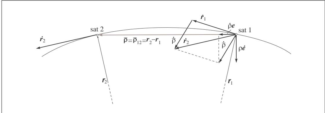
**Figure A.1.:** Position difference  $\bar{\rho}$ , range  $\rho$ , differential velocity  $\dot{\bar{\rho}}$  and range rate  $\dot{\rho}$ .
