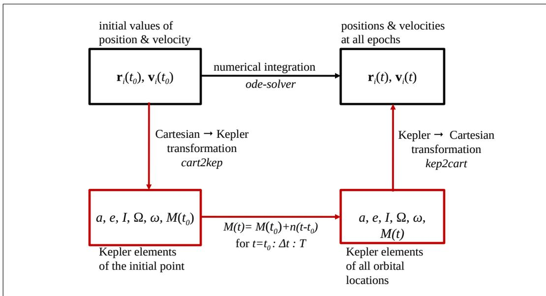
**Figure 1.1.:** Orbit propagation of a Kepler orbit based on initial position and velocity.
