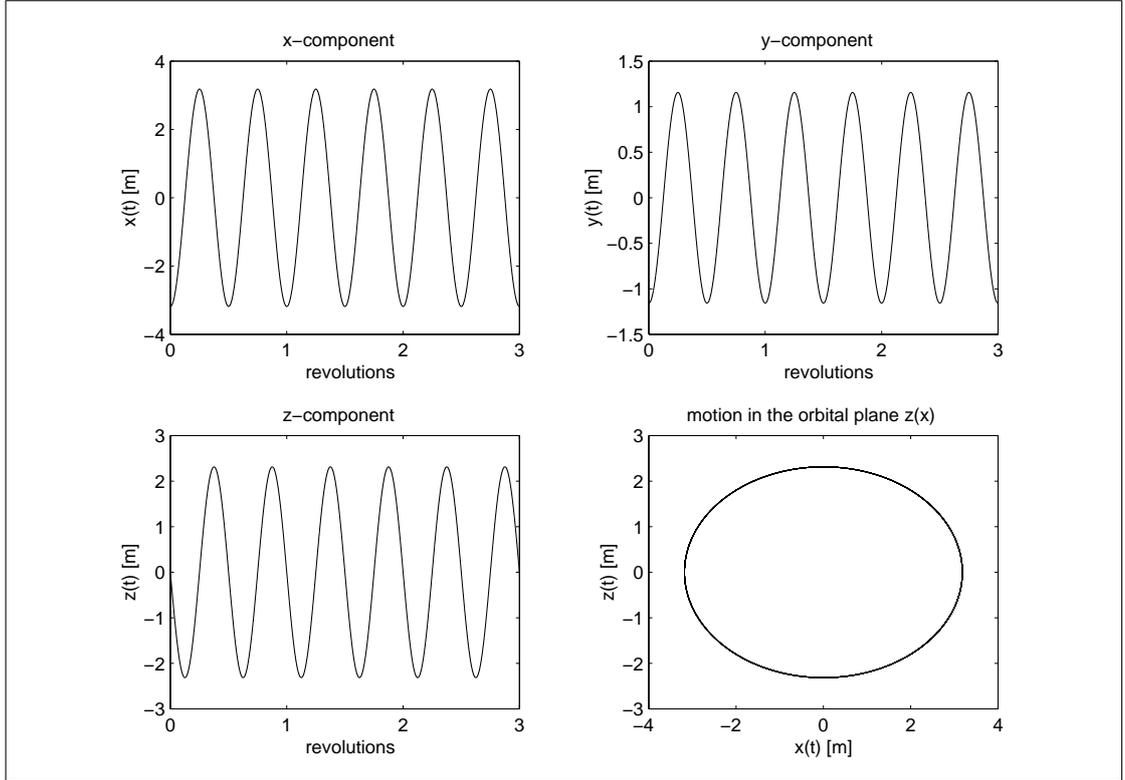
**Figure 8.3.:** Particular solution with disturbance at  $\omega = 2n$ .
