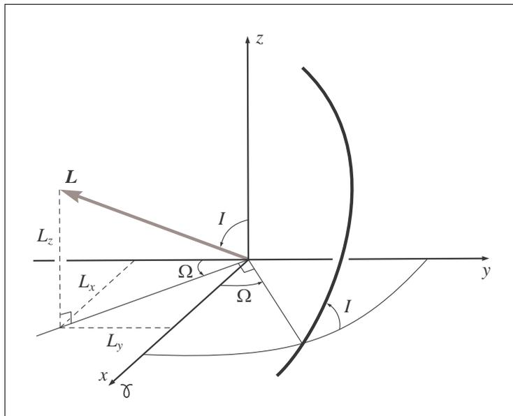
Figure 2.15.: The angular momentum vector  $L$  defines the orientation of the orbital plane in terms of  $\Omega$  and  $I$ .
