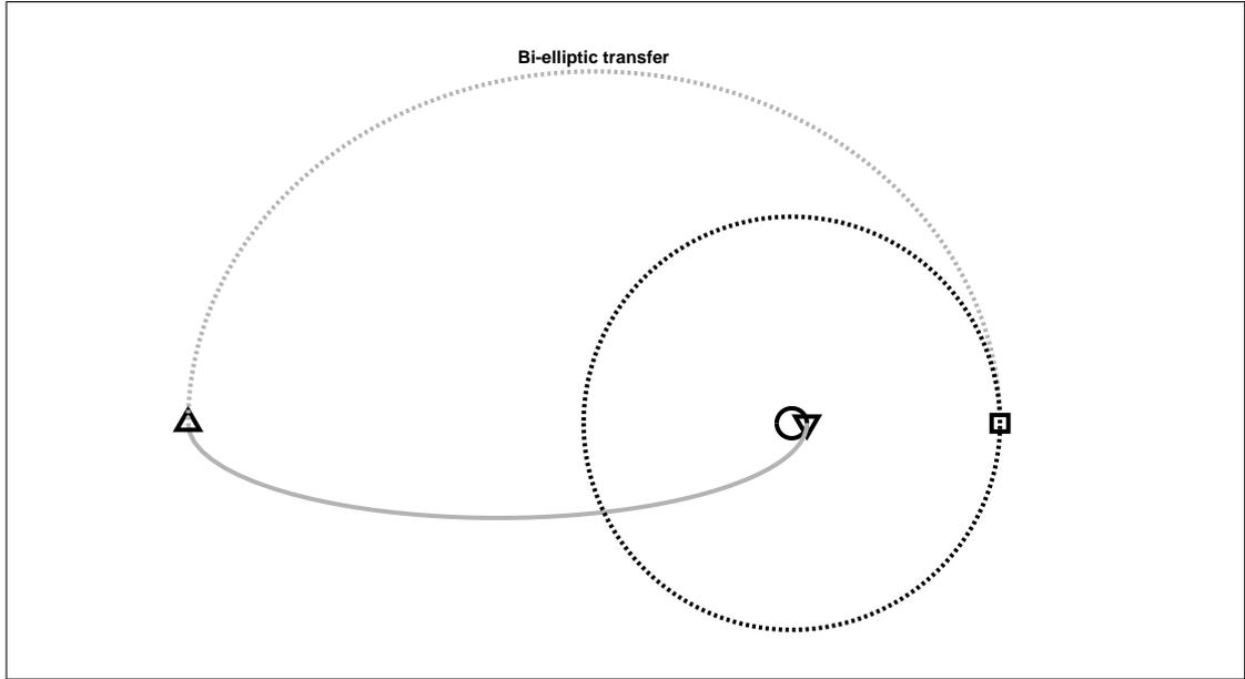
**Figure 2.13.:** Bi-elliptic transfer (in gray) between two circular orbits (in black).
