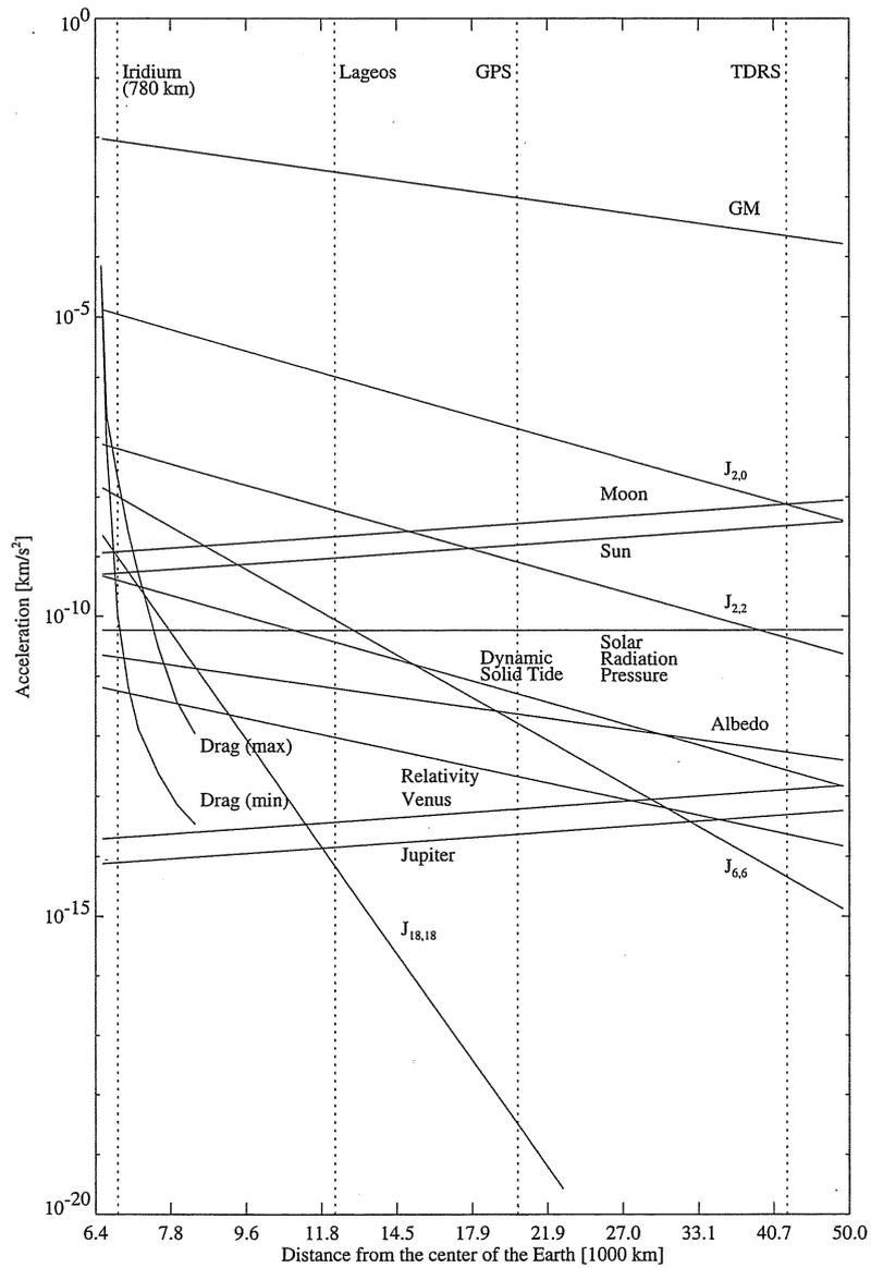
**Figure 3.1.:** Order of magnitude per orbit perturbation type in different orbital heights (Montenbruck and Gill, 2001, p. 55).
