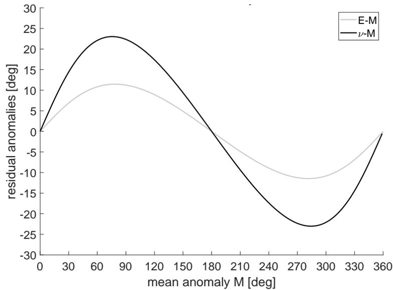
**Figure 2.10.:** Differences of the anomalies  $E - M$  and  $\nu - M$  for an ellipse with the eccentricity  $e = 0.2$ . The three anomalies coincides only in perigee and apogee, and the values differ up to  $20^\circ$ .
