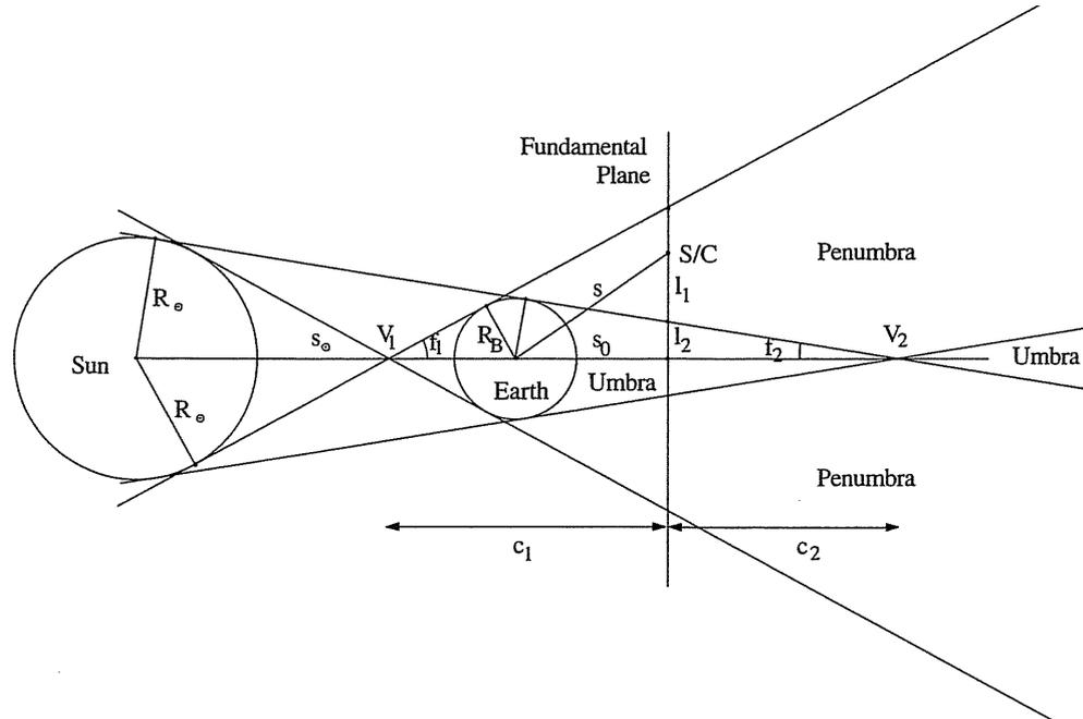
**Figure 5.3.:** The shadow function is derived via a geometrical model (Montenbruck and Gill, 2001, p. 80).
