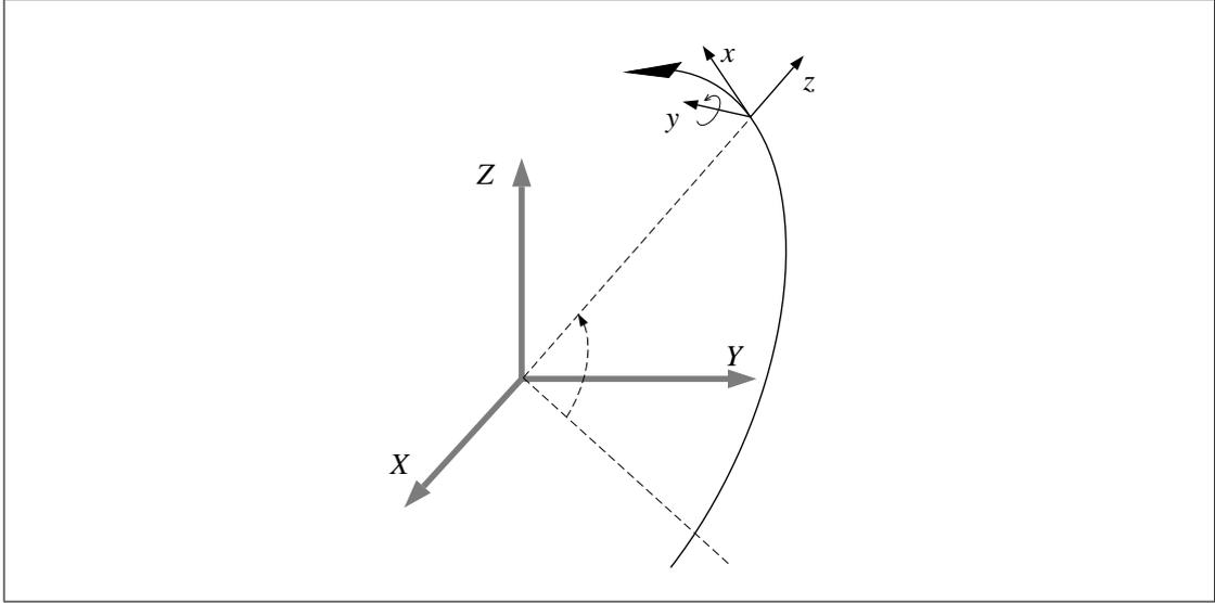
**Figure 8.1.:** The local orbital triad:  $x$  along-track,  $y$  cross-track and  $z$  radial.
