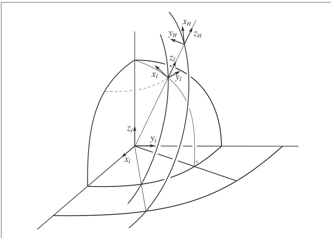
**Figure B.1.:** Coordinate systems in satellite geodesy.
