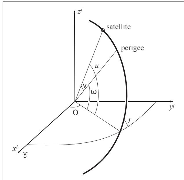
perigee  $\omega$  is counted from ascending node to perigee. The sum of angle of perigee and true anomaly is referred to as *argument of latitude*:  $u = \omega + \nu$ . This is a useful angle for circular and near-circular orbits for which the perigee is not or weakly defined.
