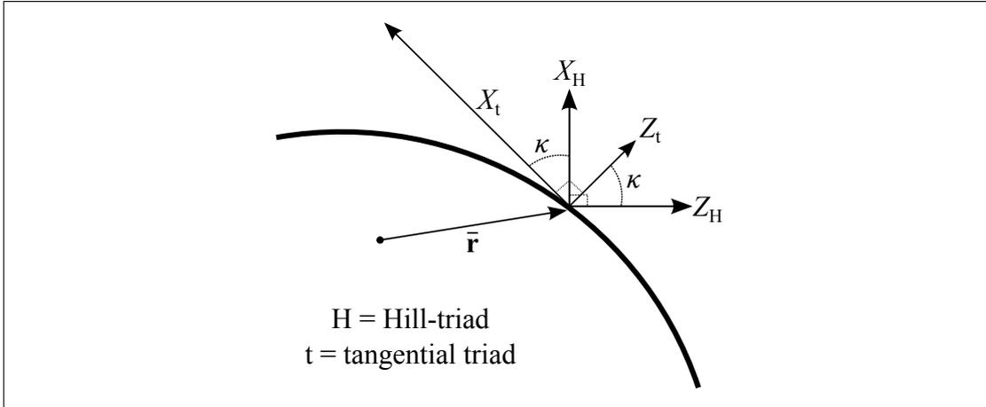
**Figure 3.2.:** Hill-triad H, tangential triad t.
