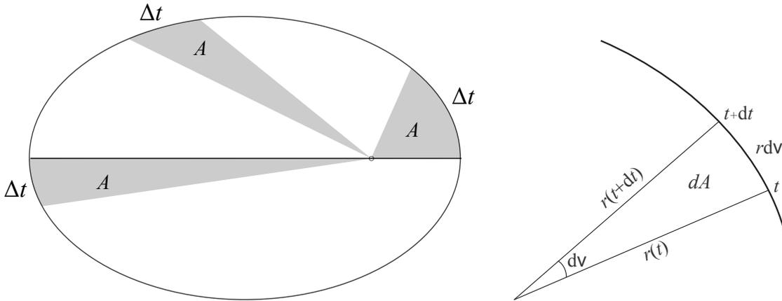
**Figure 2.3.:** Kepler's area law (left) and infinitesimal area (right).
