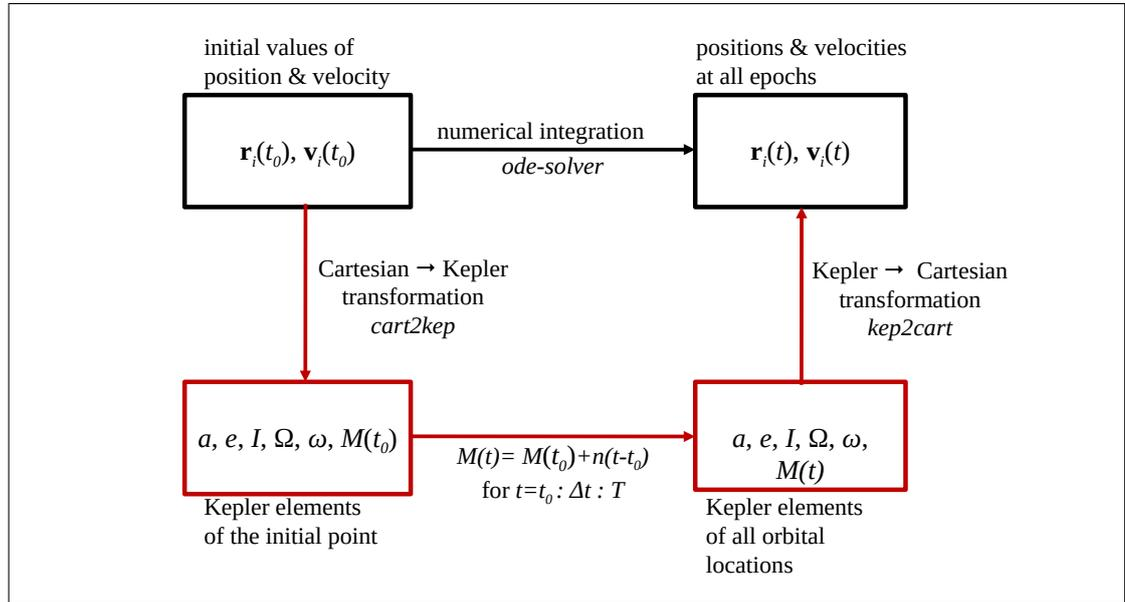
**Figure 2.9.:** Determination of a Kepler orbit based on initial positions and velocity.
