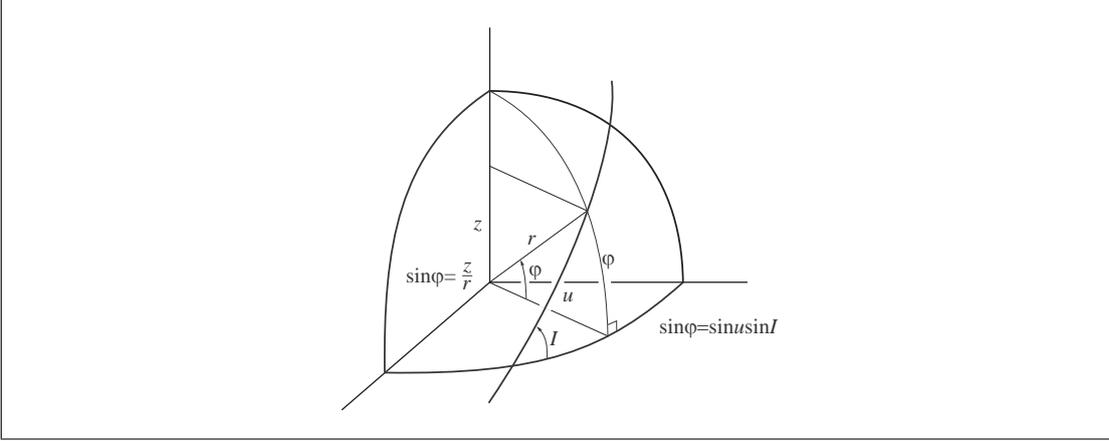
**Figure 4.2.:** Relation between latitude  $\phi$  and the Kepler elements  $I$  and  $u$  in a spherical triangle.
