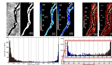
**Figure 5:** An example of probabilistic water mask. (a) is the original image, (b) is the derived water mask. (c) and (d) are the probabilistic map of the water mask and the background. The percentage shows the level of confidence to the label
