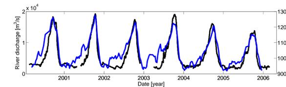
**Figure 8:** Comparison between water area time series and in situ river discharge
