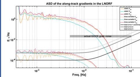
Fig. 3 Square-root of the PSDs of the static and variable part of the gradients along the orbit and requirement on the error degrading the final gradients used in the gravity field recovery.
