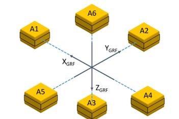
Fig. 2 Star configuration of the gradiometer, composed of 3 pairs of accelerometers.
