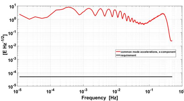
Fig. 1 Amplitude Spectral Density of the common mode accelerations and the required common mode rejection
